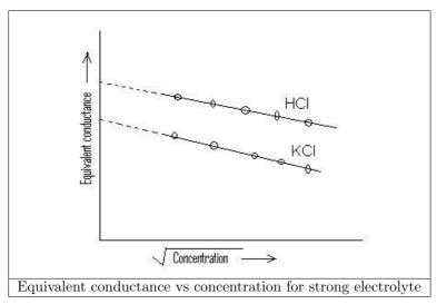
The relationship between concentration of any electrolyte and its equivalent conductance is given by Debye-Huckel-Onsagar equation:
